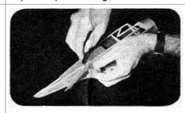
11. Cover the remaining open areas but be sure to keep the openings for the wing and stabilizer uncovered. These openings will have the wing and tail glued over them so there isn't any reason for covering them. Trim the edges right along the longerons or corner strips as shown. If you trim the piece to size before you attach it, you'll soon find it hard to do. So, always do the trimming right on the model--this is the correct way.
